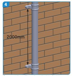
Carry on installing pipes in this fashion until reaching the drain. Clips to be fixed with plastic wall plugs and stainless steel screws of a size suitable for the substrate.
