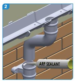
Sealant can be applied to the inside of the pipe socket prior to installation. When fitting flushjoint downpipe, sealant can also be applied to the inside of the clip to assist in supporting the pipe.
