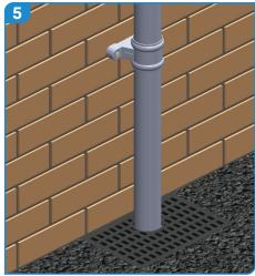
A shoe, drain adaptor or offset may be required to terminate the pipe work into the gully
