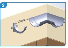
Image 2 shows the ideal bracket positioning for the angle and bracket to take the gutter length. (Max 150 mm from joint).
