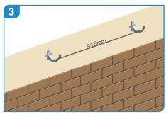
We recommend fixing brackets every 915mm and using an additional bracket for each outlet or angle.
