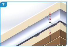
Push bolt through the sole of the gutter socket ensuring that the slot is filled with sealant before applying nut and washer, gently tighten. Do not overtighten as this may force the sealant out of the joint.
