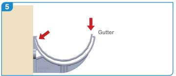
When fitting outlets and angles position the rear face of the gutter underneath the roof finish. Locate the gutter into the fascia bracket and then clip the front edge down into position.
