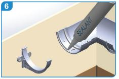
Ensure that all fixing surfaces are clean and dry. Apply 2 x 6mm beads of low modulus sealant into the socket end of gutter, place gutter length into sealant/socket.
