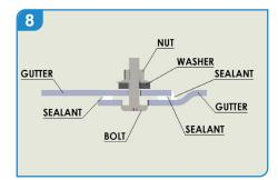
Clean off any excess sealant to either side of the joint. Apply additional sealant as required to the internal face only to create a smooth bead.
