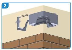
Image 2 shows the bracket for the angle and a bracket to take the gutter length.
