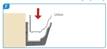
After sealant is applied to gutter surfaces place union over joint and press down firmly until the union clips into place on both front and rear face of the gutter.
