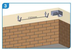
We recommend fixing brackets every 750mm and using an additional bracket for each outlet or angle. Ideally using a string line or laser level between the two brackets, set out intermediate brackets at maximum centres of 750mm.
