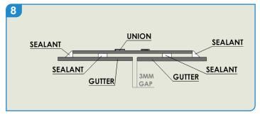
Clean off excess sealant along the edges of the joint. Use the same process for every joint until the work is completed
