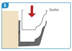
When fitting outlets and angles tuck the rear face of the gutter underneath the roof finish. Locate the gutter into the fascia bracket and then press down into position.
