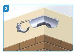
Image 2 shows the bracket positioning for the angle and bracket to take the gutter length.
