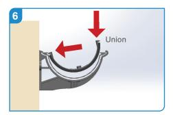
Ensure that all fixing surfaces are clean and dry. Placing the union into the groove in the rear face of the gutter and clip down into place on the front edge.
