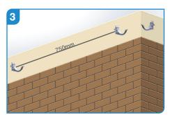
We recommend fixing brackets every 750mm and using an additional bracket for each outlet or angle. Ideally using a string line or laser level between the two brackets, set out intermediate brackets at maximum centres of 750mm.
