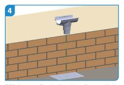
With the use of a plumb or laser line, position outlets over gullies and support with at least one bracket. Also include a bracket per angle (internal or external).
