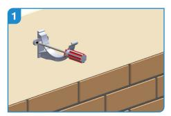
Start by deciding whether to fit the gutter level or with a fall to 1:600. Fit a bracket at each end of a run. Position brackets correctly for an angle or stopend.
