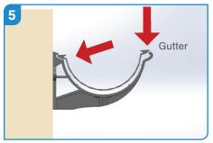
When fitting outlets and angles tuck the rear face of the gutter underneath the roof finish. Locate the gutter into the fascia bracket and then clip the front edge down into position.
