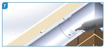
Trim 4-5 mm off top of nozzle so it fits snuggly into the large holes in the base of the union, inject the special\* low modulus sealant supplied into one of the large holes in the bottom of the union until the sealant appears at both of the smaller holes at the rim of the union. Repeat the action on the other large hole. (\*Sealant only available from ARP).
