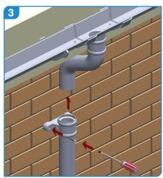
Additional pipe clips should be fitted at 2m maximum intervals.
