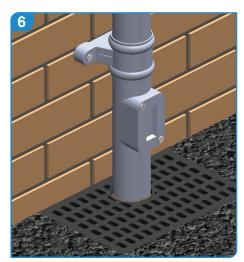
As per local building regulations, if a shoe is not installed access pipes should be fitted and positioned to give suitable rodding access as required.
