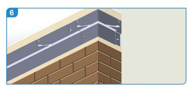
Apply nuts and washers and gently tighten (Do not overtighten as this may force the sealant out of the joint).
