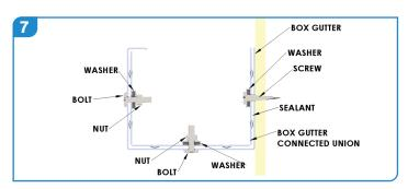
Clean off any excess sealant to either side of the joint or apply additional as required to create a smooth bead.
