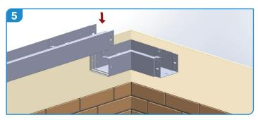
Position the spigot end over the joint, push bolts through the slots of the gutter from the outside, making sure the slotted holes are filled with sealant.
