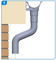
Ensure vertical alignment between drain and gutter outlet.
