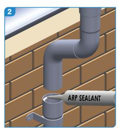
Sealant can be applied to the inside of the pipe socket prior to installation. Swaged and flushjoint downpipes should have sealant applied to the socket prior to installation. Cast Collared can be sealed after fitment. When fitting flushjoint downpipe, sealant can also be applied to the inside of the clip to assist in supporting the pipe.
