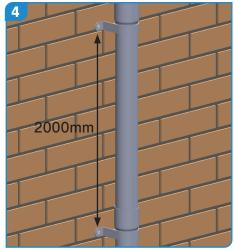
Additional pipe clips should be fitted at 2m maximum intervals.
