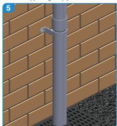
A shoe, drain adaptor or offset may be required to terminate the pipe work into the gully
