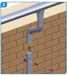
A pipe clip should be fixed directly beneath the pipe socket.
